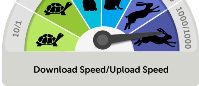
The diagram above shows how most internet providers list speeds. **Download speed**, the number on the left, is the speed that information on the Internet (e.g., text and graphics) is transferred to your computer; that is, how
